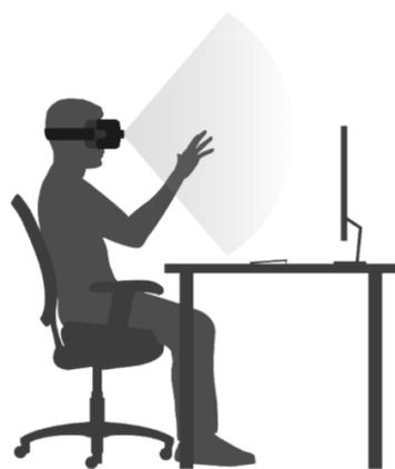
The Leap Motion Controller features a 120x150° field of view and an interactive tracking range of more than 2 feet (60cm).
