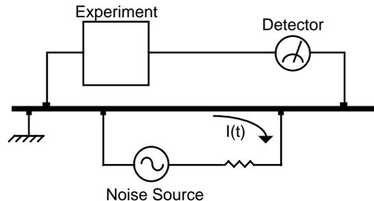
In this illustration, the detector is measuring the signal relative to a ground far from the rest of the experiment. The experiment senses the detector signal as well as the voltage from the noise source's ground return current, which passes through the finite resistance of the ground between the experiment and the detector. The detector and the experiment are grounded at different places which, in this case, are at different potentials.
