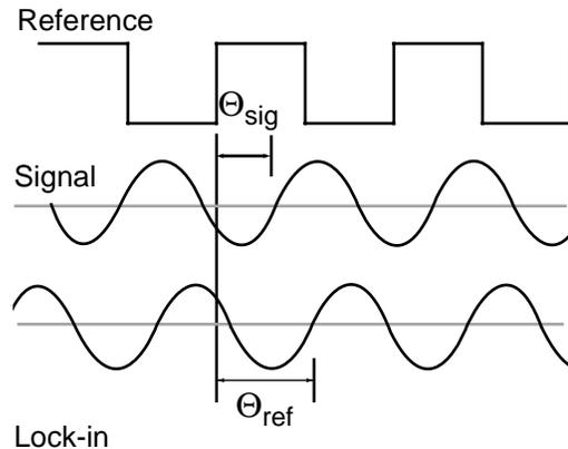
The lock-in amplifies the signal and then multiplies it by the lock-in reference using a phase-sensitive detector or multiplier. The output of the PSD is simply the product of two sine waves.
